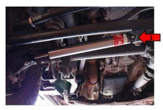
Step 6. Install the Eibach steering damper onto the vehicle with the body of the damper facing the driver's side. Be sure to have the Schrader valve face the front of the vehicle (1).
