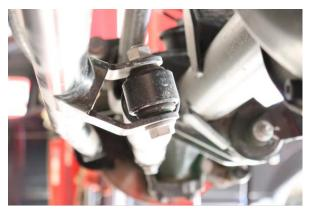
Step 2. Remove 18mm bolt & nut from driver side of OE damper.
