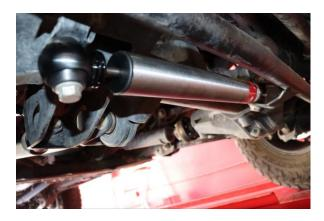
Step 9. Check that the steering wheel can reach full extension left and right without binding. Shown above damper at full right turn.
