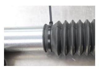
Step 4. Install dust boot over damper shaft, tighten cable tie to bottom of tube. Trim off excess cable.
