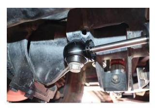
Step 7. Install and tighten 18mm steering damper bolt to manufacturer specifications.
