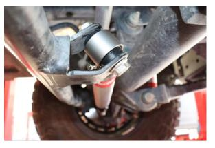
Step 8. Install 18mm bolt and nut securing the rod end of the steering damper to the bracket. Tighten steering damper bolt to manufacturer specification.
