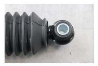
Step 5. Install dust boot cover onto damper end; insuring rubber seats into groove.
