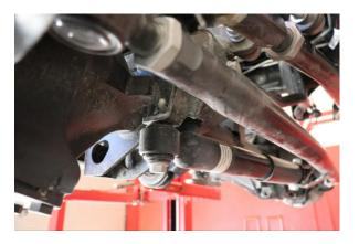
Step 3. Remove the 18mm bolt securing the steering damper from passenger side. Be aware as the damper will be free. Lift up and pull towards the passenger side to remove.
